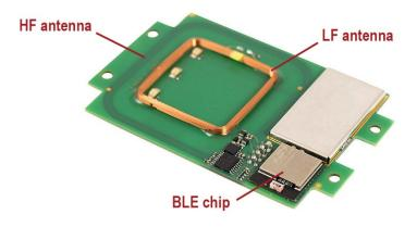
HF antenna (13.56 MHz) Dimensions: 42 x 44 mm / 1.65 x 1.73 inch Number of turns: 3
